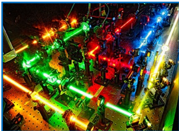
4-color laser TIRF microscopy setup in Jeff Gelles' Laboratory at Brandeis University
